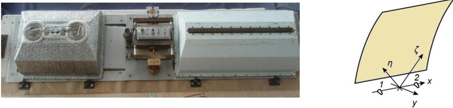
**Fig. 1.** New generation AC adjustment complex installed in the center of the movable carriage of the feed cabin No. 2 (left), coordinate system near focus (right)
