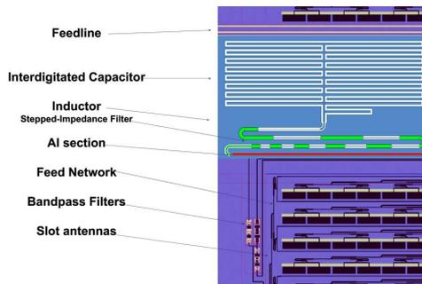
**Fig. 2.** Mask design: layout of the major components on the wafer.
