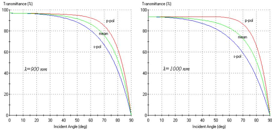
**Fig. 3.** Surface transmittance of monocrystalline silicon with HfO<sub>2</sub> quarter-wave anti-reflective layer at different angles for 900 nm and 1000 nm wavelength
