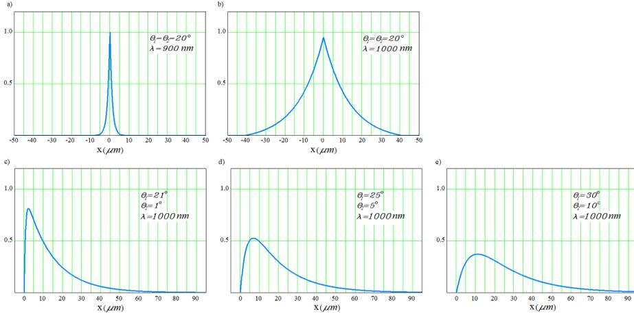
**Fig. 2.** PSF of the chromatic aberration for 900 nm (a) and 1000 nm wavelengths (b) of normal incidence light, and 1000 nm same quarter incident at different angles (c)(d)(e) for aperture equivalent to f/2.6 optical system
